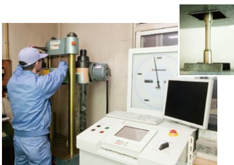
20-ton Amsler universal testing machine
